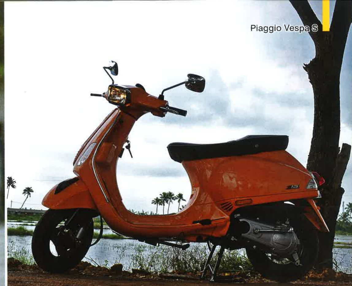
Above: Vespas are one of the few scooters that still make use of a monocoque chassis design. Below: The rear, three-quarters is the same as that of its siblings apart from the Vespa S and the S125 badging
