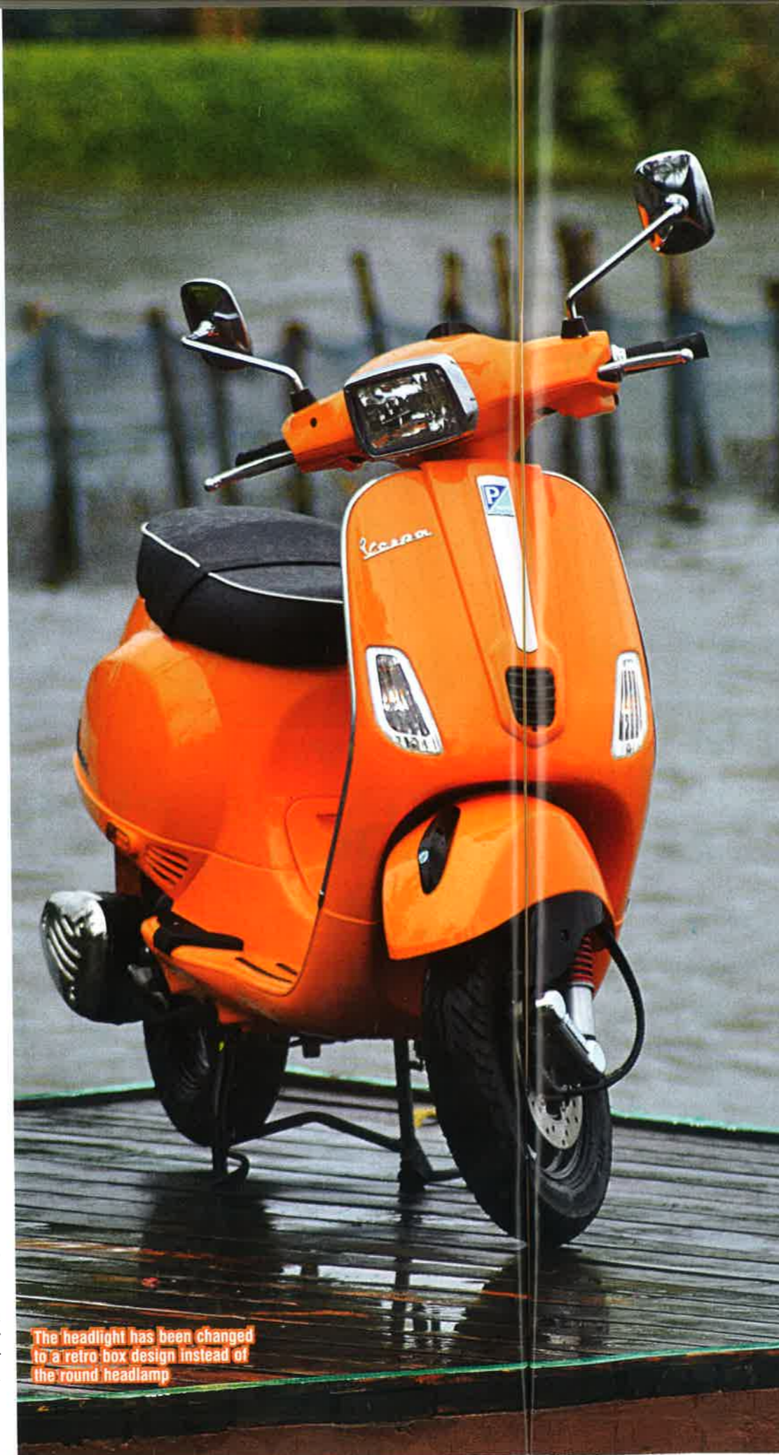
Above: Vespas are one of the few scooters that still make use of a monocoque chassis design. Below: The rear, three-quarters is the same as that of its siblings apart from the Vespa S and the S125 badging
