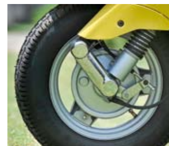
LX125 front drum brake lacks power.
